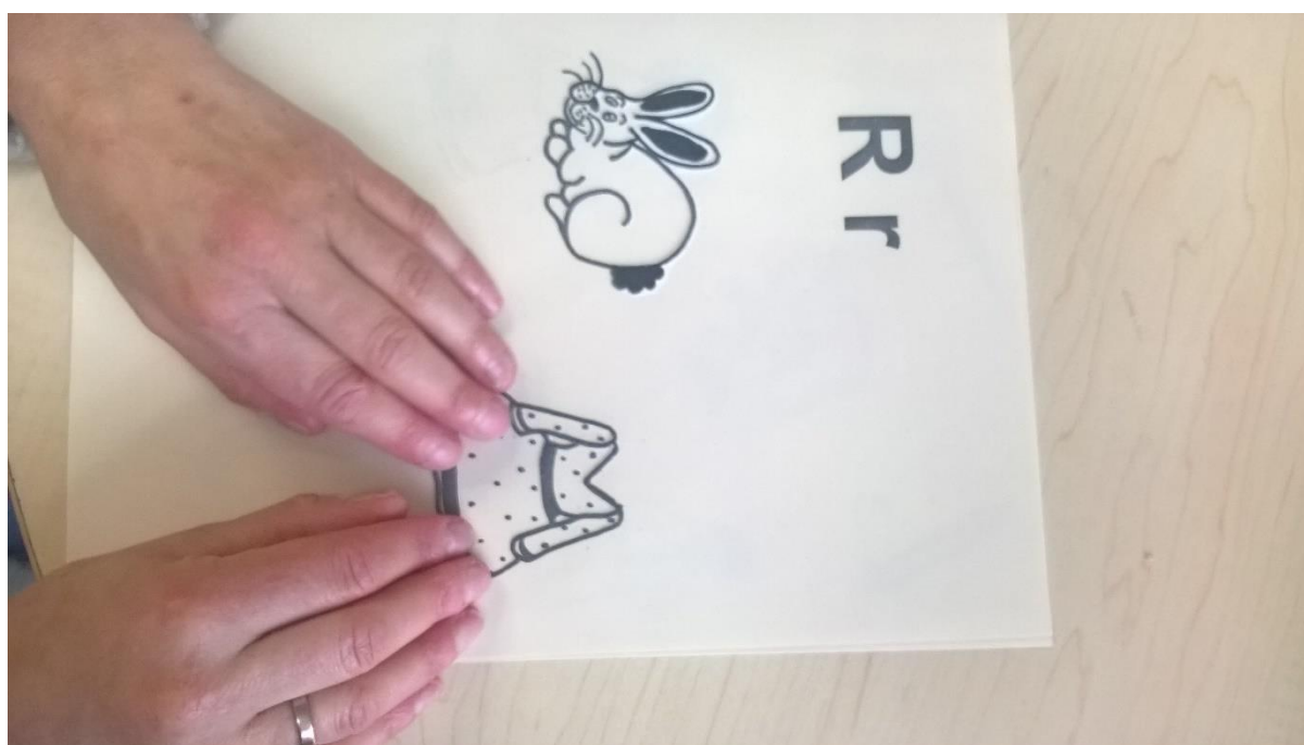
Figure 9: Close-up of swell-paper with tactile representation of letters and objects
