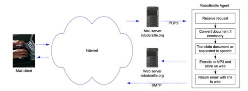
Fig. 3. RoboBraille text-to-speech translation process. From [1].
